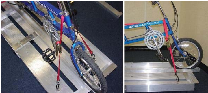
Figure 17.10. Securing of the Front Wheel
