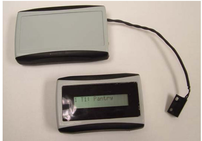
Figure 9.8. Completed Pager and Door Sensor
