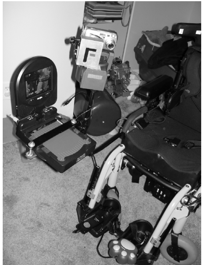
Figure 7.1. Foot-Operated Camera System, with Camera and Screen Rotated Out
