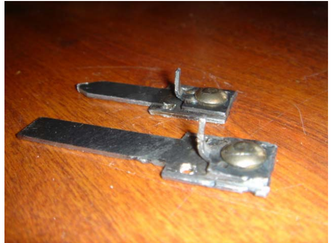
Figure 16.5. Custom Tips for Chisel (Foreground) and Nail Set (Background).
