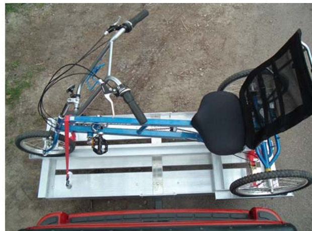
Figure 17.12. Final Trike Racking System (Top View)
