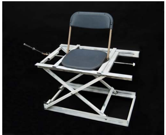
Figure 11.57. Adjustable Scissor Lift in Raised Position
