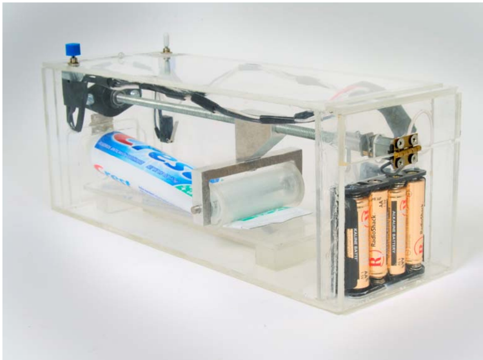
Figure 11.24. Hinged Access Door to Batteries and Motor
