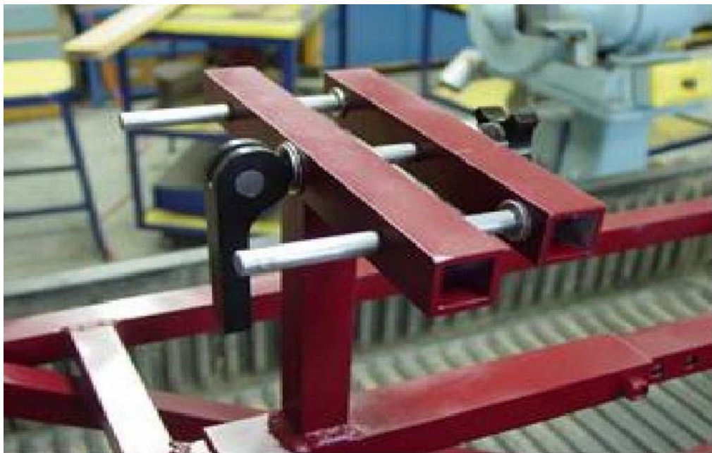
Figure 14.19. Clamping Mechanism to Hold Wheelchair
