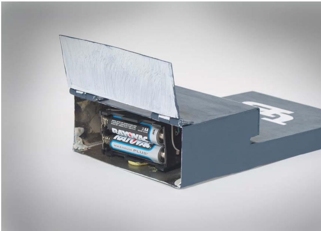
Figure 11.29. Hinged Door of Battery Compartment
