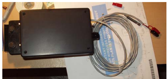
Figure 15.8. LP Digital Interface and Mounting Platform
