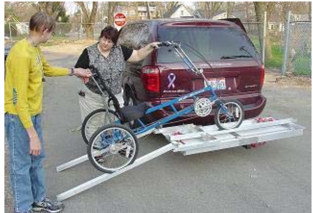
Figure 17.1. Client (on left) Testing Trike Racking System
