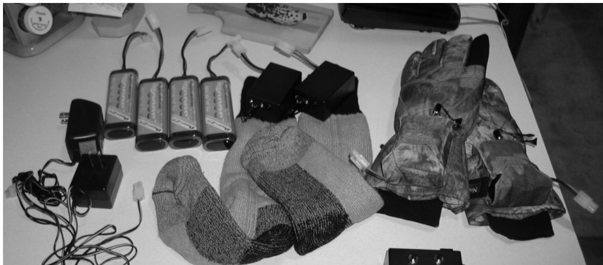
Figure 15.23. Socks and Gloves with Devices Attached, with Batteries and Control Box
