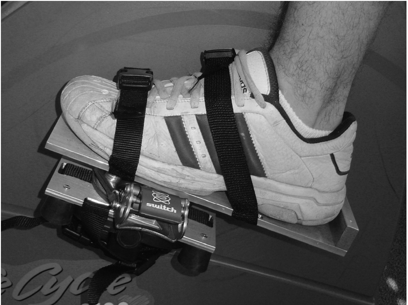
Figure 6.4. Adaptor for Exercise Bicycle Pedal, Attached to Existing Pedal
