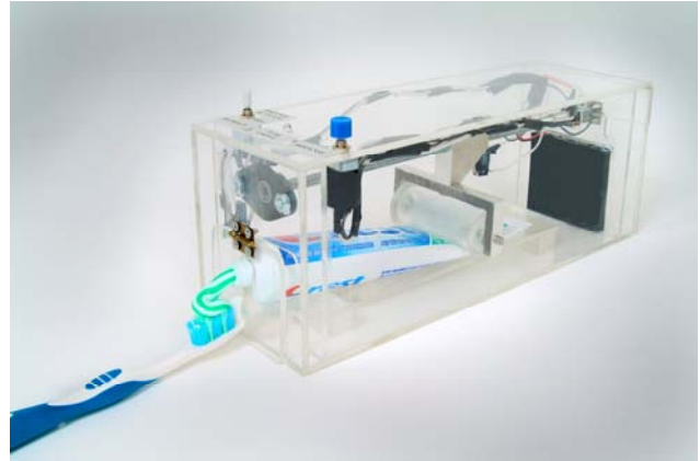
Figure 11.22. Battery Operated Automatic Toothpaste Dispenser
