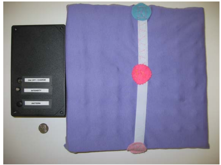
Figure 9.14. Completed Vibrotactile Stimulation Pad
