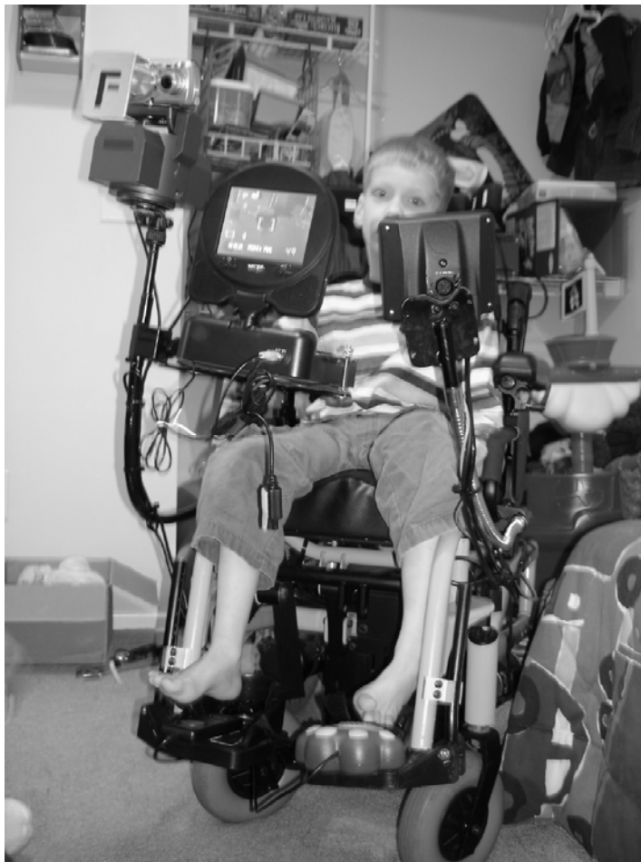
Figure 7.2. Client Using Foot Operated Camera, with LCD Screen Rotated 180 degrees
