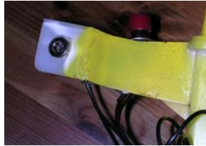
Figure 12.10. Female Power Adapter for Soap Pump
