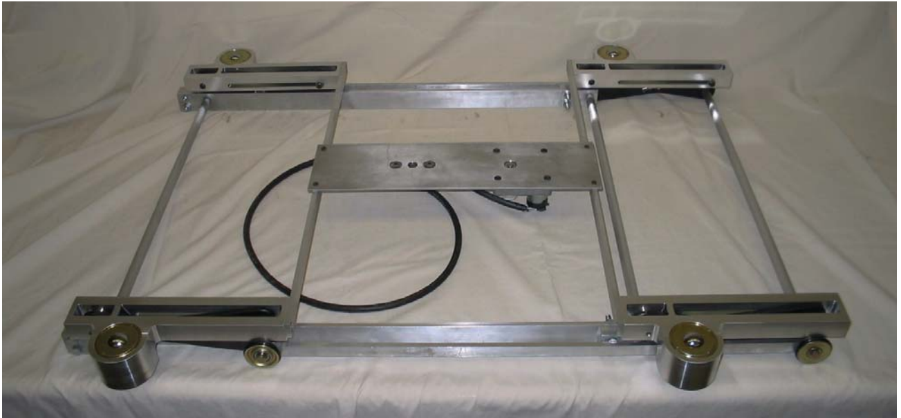
Figure 19.20. Base Assembly And Legs/Lifting Assembly in Fully Down Position
