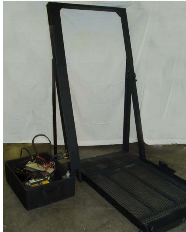
Figure 8.1. Modified Van Lift with Box Containing Hydraulic Motor and Battery
