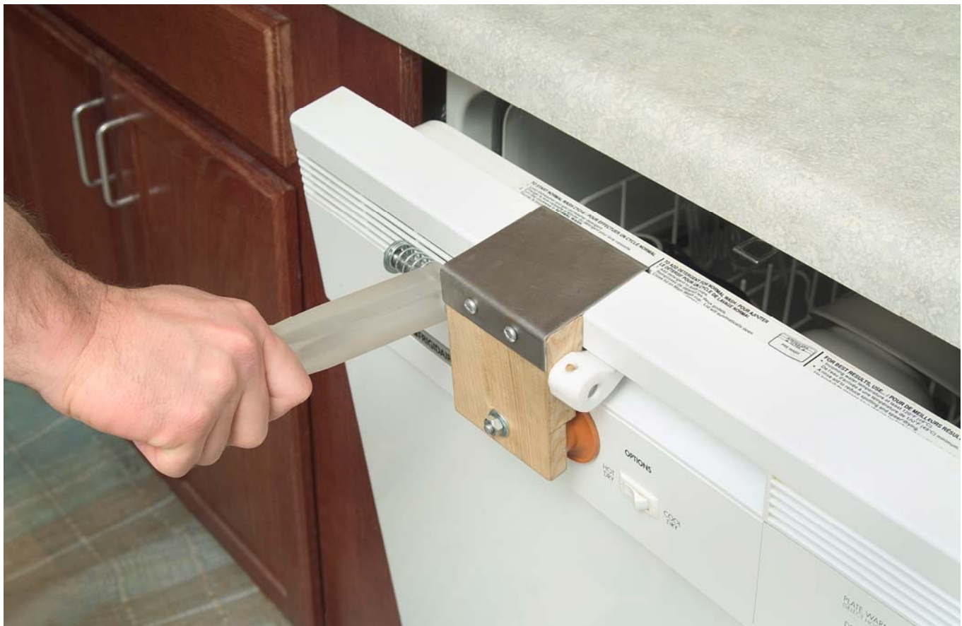
Figure 11.13. Lever-Operated Dishwasher Opener in Use
