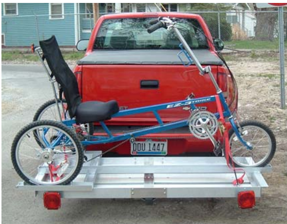
Figure 17.11. Final Trike Racking System (Rear View)
